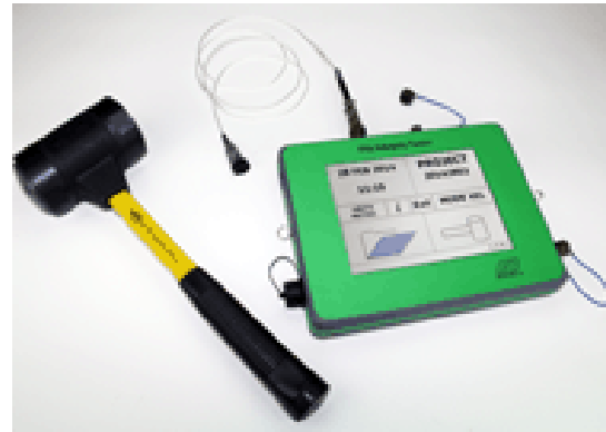
PIT test equipment
