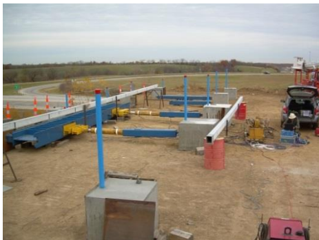
Static lateral test of pile
